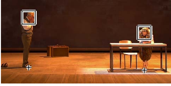
Figure 2: Input to the system are the upper body bounding boxes for each actor (shown with squares) and the points where the actors touch the stage floor (shown with cross markers).
