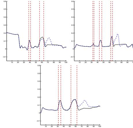
**Figure 21:** Profiles through the hot structure for the case without truncation. The profiles for the horizontal, oblique, and vertical lines are top left, top right and bottom figure, respectively. The plain black line is the reconstruction of the activity without the hot-spot and the dashed blue line is the one with the hot spot.
