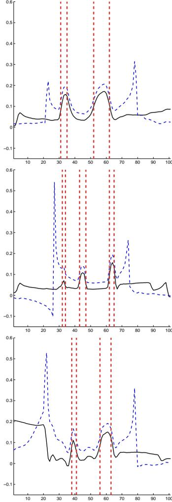
**Figure 16:** Sampling along the horizontal is green profile (at the top), along the diagonal is the yellow profile (picture in the middle) and along the vertical is the blue profile (bottom). The black line is the reconstructed counts for the attenuation but non truncated case and the blue dashed line shows the reconstruction of the attenuated truncated projections. The dashed red lines are the limits of the heart wall.
