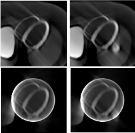
**Figure 20:** Effect of the hot spot. The pictures on the top show the results for the non truncated case. The left figure is the reconstruction without the hot spot and the right figure is the reconstruction with the hot spot. In the same order, the pictures on the bottom show the reconstruction for the truncation case.
