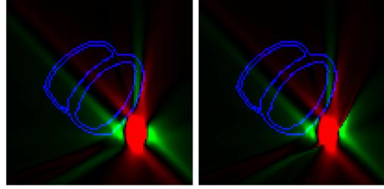
**Figure 24:** Error map for the effect of the hot structure on the entire surface. The figure on the left shows the difference due to the hot spot in the non truncation case. The figure on the right is for the truncation case. The red color is an increase of counts due to the hot structure while the green color is a decrease.
