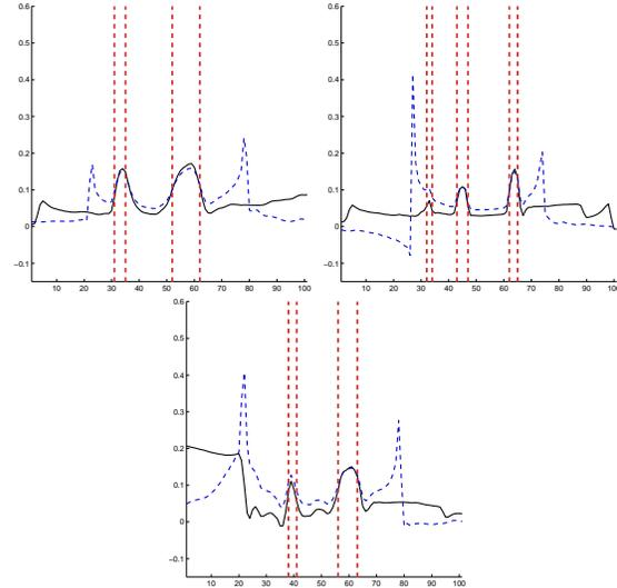
**Figure 18:** Samples for the corrected case with a scaling factor  $\mu = 0.77$ . Horizontal is the green profile (first picture), diagonal is the yellow profile (picture in the middle) and vertical is blue profile (bottom picture). The black line is the reconstructed counts for the attenuation but non truncated case and the blue dashed line shows the reconstruction of the attenuated truncated projections. The dashed red lines are the limits of the heart wall.
