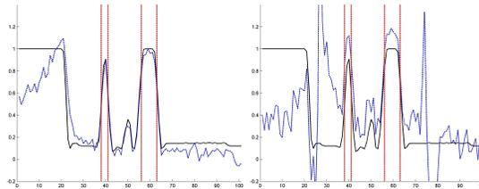
**Figure 31:** Sampled profiles of the algebraic reconstruction. The black line is the true value and the dashed blue line is the reconstructed value. The vertical red lines are the boundaries of the heart wall. The picture on the left is the results for the least square reconstruction. The results on the right are the reconstruction for the ART reconstruction.
