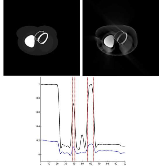
**Figure 14:** Comparison between non attenuated (top left) and attenuated (top right) reconstruction of the activity distribution. In the figure on the right, the intensity is scaled by a factor of 3.8. The figure at the bottom shows a profile of samples of counts for the non attenuation case (black) and for the attenuation case (blue).
