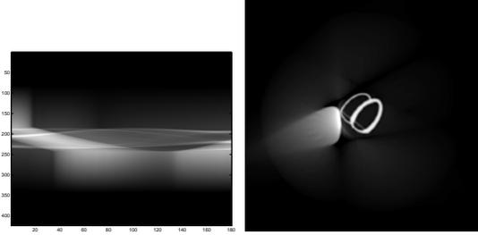
**Figure 26:** The ring effect is suppressed by linear interpolation of the values of the sinogram between the limit of the boundary to zero. The picture on the left is the sinogram and the picture on the right shows the reconstruction without the ring artifact.
