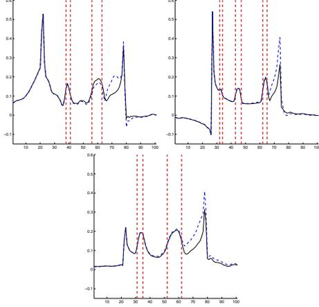
**Figure 22:** Profiles through the hot structure for the case of truncation. The profiles for the horizontal, oblique, and vertical lines are top left, top right and bottom figure, respectively. The plain black line is the reconstruction of the activity without the hot-spot and the dashed blue one with the hot spot.
