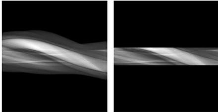
**Figure 5:** The picture on the left shows the complete sinogram before truncation, picture on the right shows the effect of the truncation on the projection data assuming the trajectory is perfectly circular.
