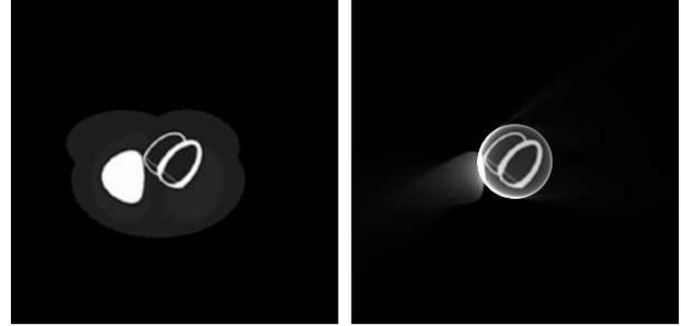
**Figure 9:** Results of the back projection of the activity map for the non attenuated case. Picture on the left is the non truncated reconstruction and the picture on the right is the results of truncation. The intensity of the truncated picture is scaled by a factor of 0.75.
