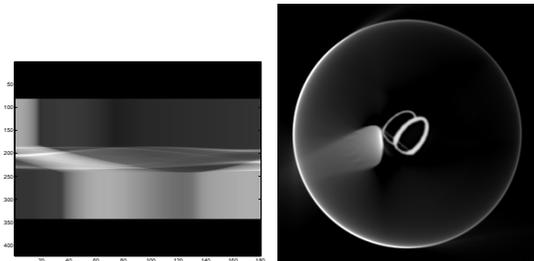
**Figure 25:** The picture on the left shows the copy of the line of the sinogram to translate the discontinuity. The picture on the right is the reconstruction where the ring effect is now far from the heart.
