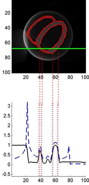
**Figure 10:** Example of sampling for the corresponding position through the heart. The black line is the sampling on the filtered backprojection reconstruction of the non truncated activity map. The dashed blue line corresponds to the truncated reconstruction and the dashed red line delineates the position of the heart wall.
