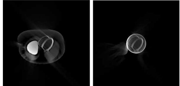
**Figure 15:** Visualization of the artifacts for the truncation case. The picture on the left shows the reconstruction of the non truncated projections. The picture on the right shows the reconstruction of the truncated projections. The intensity in the left picture is scaled by a factor of 3.7 and the intensity in the right picture is scaled by 2.50.
