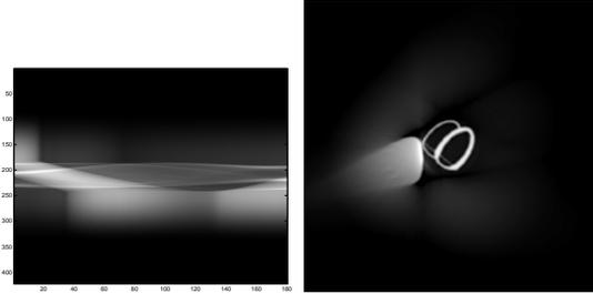
**Figure 27:** The ring effect is suppressed by interpolation with a cosine function for the values of the sinogram between the limit of the boundary to zero. The picture on the left is the sinogram and the picture on the right shows the reconstruction without the ring effect.
